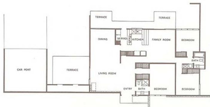
Figure 4:16 Plan B from Living Conditioned Homes in Northridge is a version of the “Extrovert” plan with family room and children’s bedrooms in one separate zone. Living Conditioned Homes by Sanford D. Adler, Photographs, drawings and tract brochure reproductions used herein are from William Kriese’s personal collection and are used by permission of William Kriese, AIA-E, Architect.
