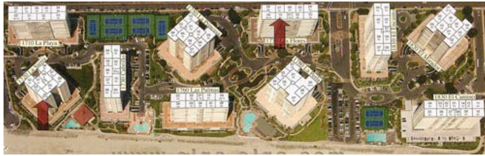
Figure 4:32 As-built plan of Coronado Shores after Coastal Commission requested changes to original plan. Note slight alteration to placement of three buildings at right to accommodate access road and public parking lot. Angles and view corridors were maintained in the revised plan. Photographs, drawings and tract brochure reproductions used herein are from William Krisel's personal collection and are used by permission of William Krisel, AIA-E, Architect.
